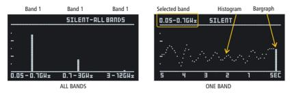
**AUDIO** – the 1216 produces the signal's audio footprint. Some signals have a typical sound, for example, a Wi-Fi or mobile GSM/3G/LTE device, so the user can recognize the protocol in some cases. The joystick's  $\blacktriangleleft$  and  $\triangleright$  buttons can be used for selecting the band
